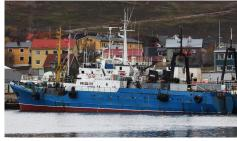
Additional details: The vessel was built with SRTMk-type (mid-sized freezing stern trawler) hull utilized. It's completely prepared for crab fishery. Powerful RSW-chiller and air compressors. Fuel consumption: 2.8 - 3.5 t per day for 6 - 14 knots speed.
